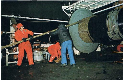
The present streamer concept allows the use of up to 114 hydrophone groups with various spreads.
