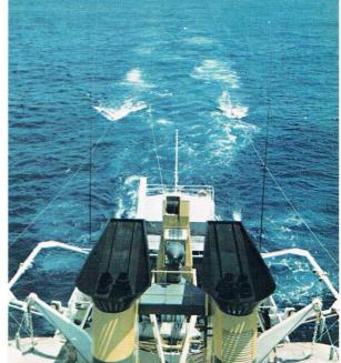
**Tuned airgun arrays** serve as energy source. Synchronous operation of all airguns is achieved by an automatic ▲ release control system.
