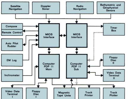
Navigation and positioning: PRAKLA-SEISMOS's INDAS V, an abbreviation of Integrated Navigation Data Aquisition System, is the concept the company has put into service to maintain highest positioning standards, including quality controls.
