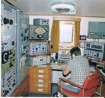
**Worldwide communication** is established by comprehensive radio equipment; marine LW, MW and SW transcoms also in SSB mode, all marine VHF channels, radio telex and weather chart printer.
