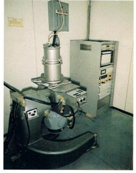
The seismic recording instrumentation is the principal constituent of any seismic survey vessel. The most up to date digital field recording units provide a recording capacity of up to 120 seismic channels at present - a 200 channel system is scheduled for introduction in 1980.
