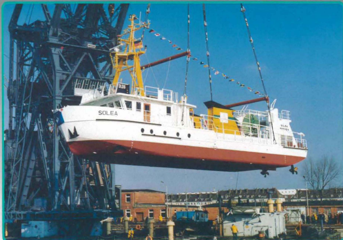
The launching lift of the research ship 'Solea' (a shallow water vessel) by the MWB floating crane
