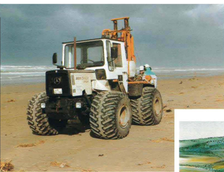
Light drilling rig P 0501
