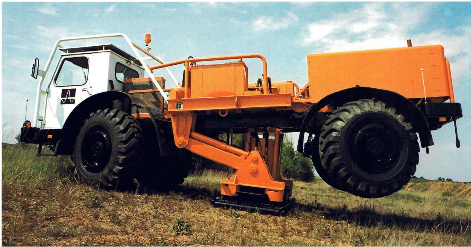
The vibrator type VVCA is an all terrain vibrator approved and equipped for driving and vibrating in european countries but can also be equipped to suit the regulations in other countries with desert areas or
